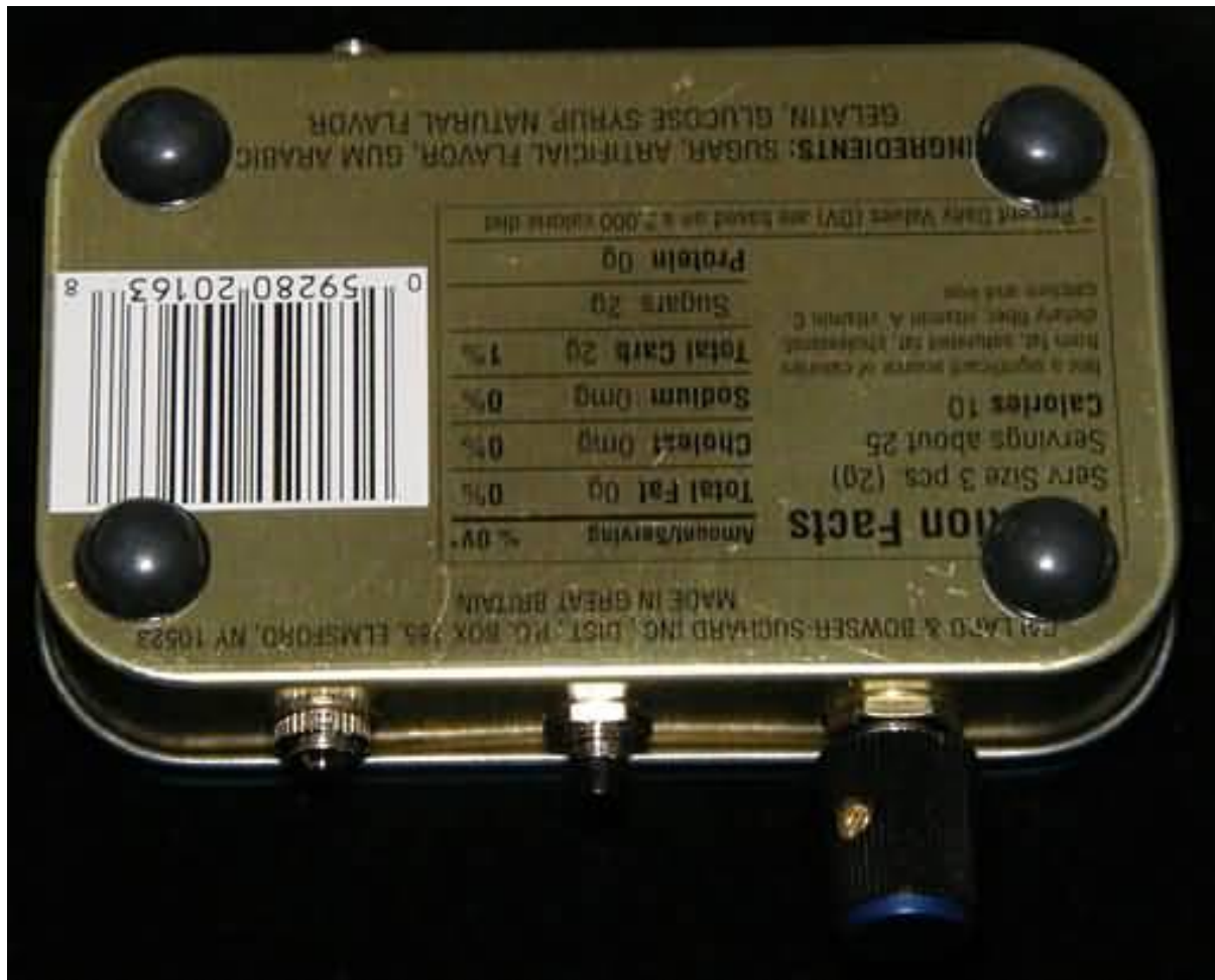
Figure 61 – Rubber feet on bottom of Altoids tin adds a nice soft touch
