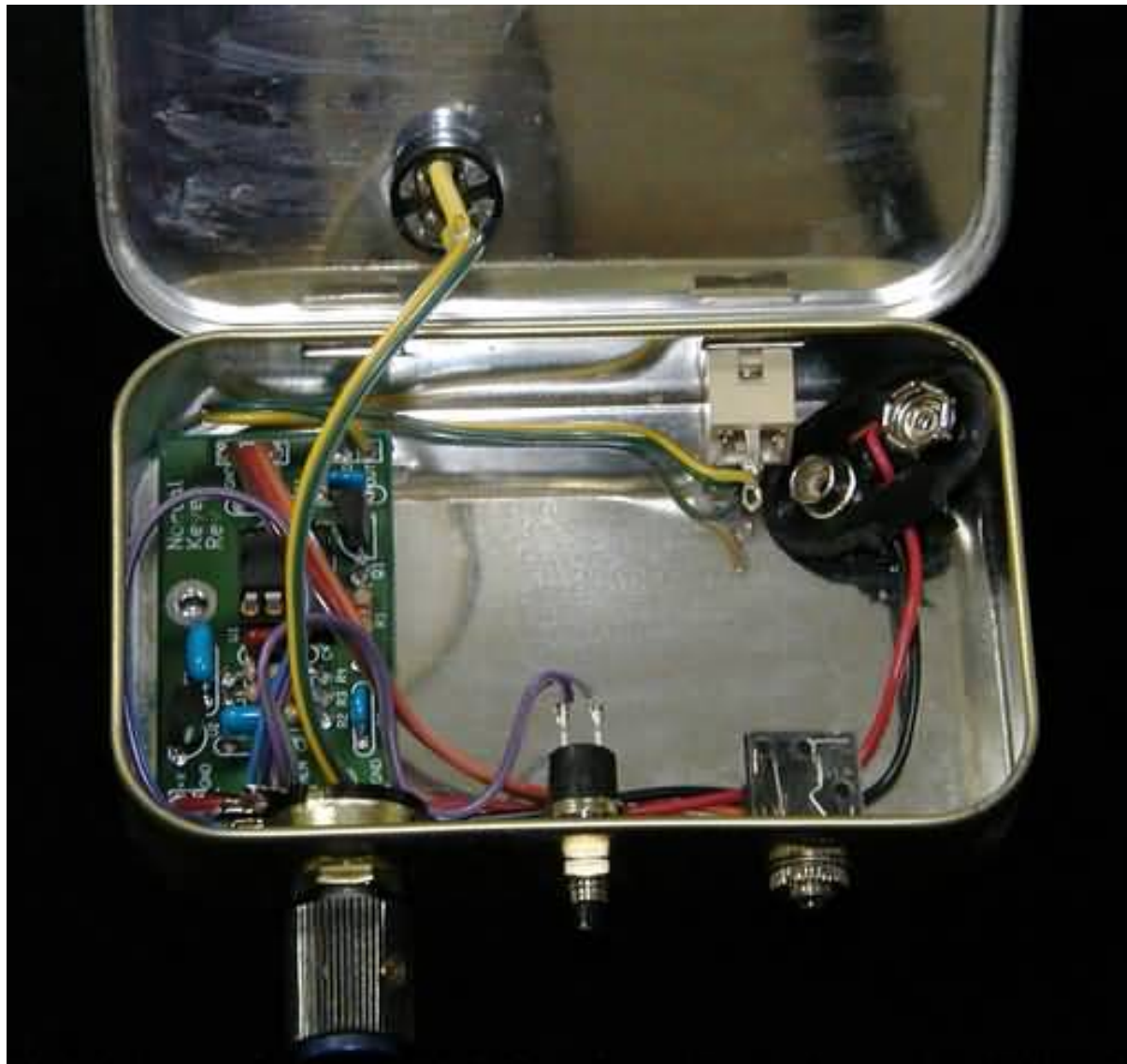
Figure 59 – inside Altoids tin showing components mounted
