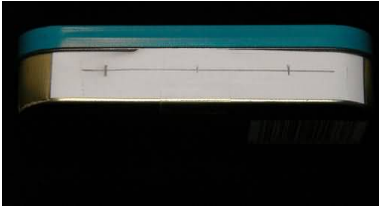
Figure 57 – Altoids tin with paper noting hole locations
