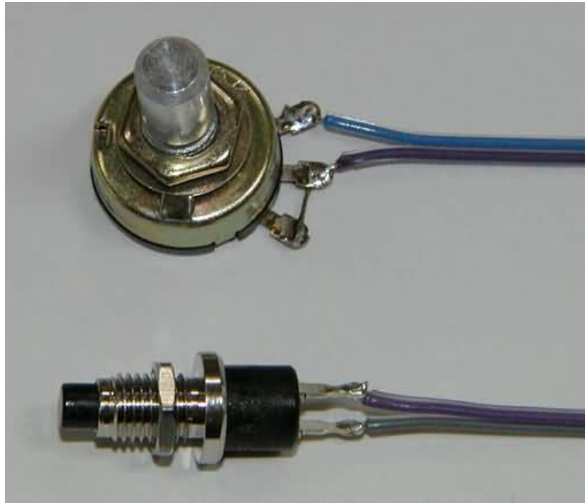
Figure 52 – Potentiometer and switch with leads attached
